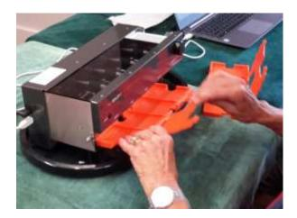
Dinah places the open board into the machine The cards automatically go into the right places as dictated by the screen, the micro chip and the camera– it's a very quick process – takes about 8 seconds to deal a hand
